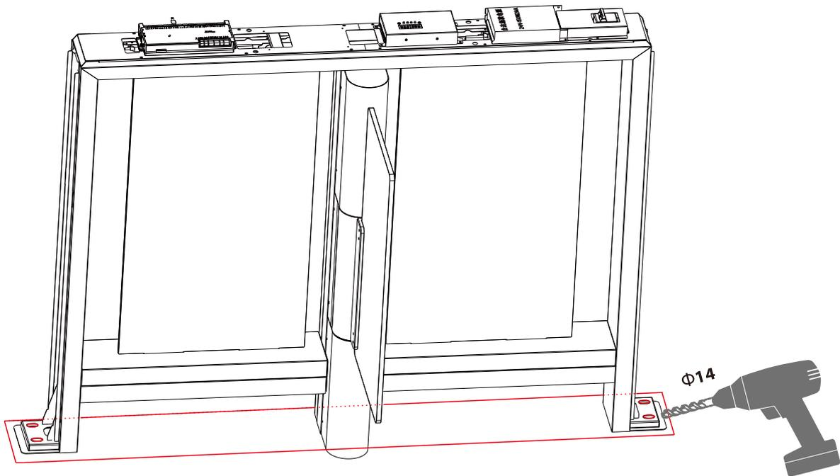
6. Clean up the soil and dust after the drilling is completed, place the turnstile to the installation site again.
